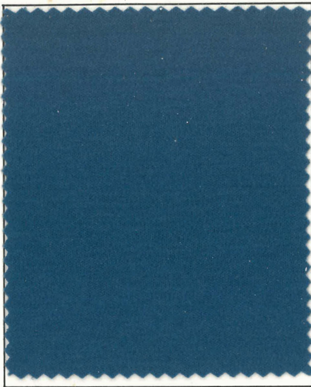
Fig. 1: 28gg/Interlock Fabric (74% Wool/26% Nylon) knitted from 16 Tex RWCS yarn spun from shrink-resist treated wool tops.
