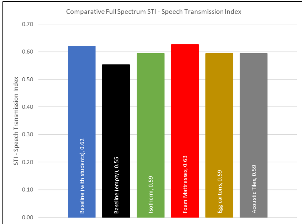
Figure 6. STI results measured for each material intervention relative to the baseline measurement(s).
