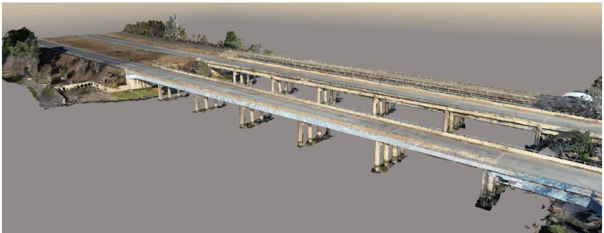
Figure 2-2: Point cloud model of strategic bridge P155_01N_B3886
