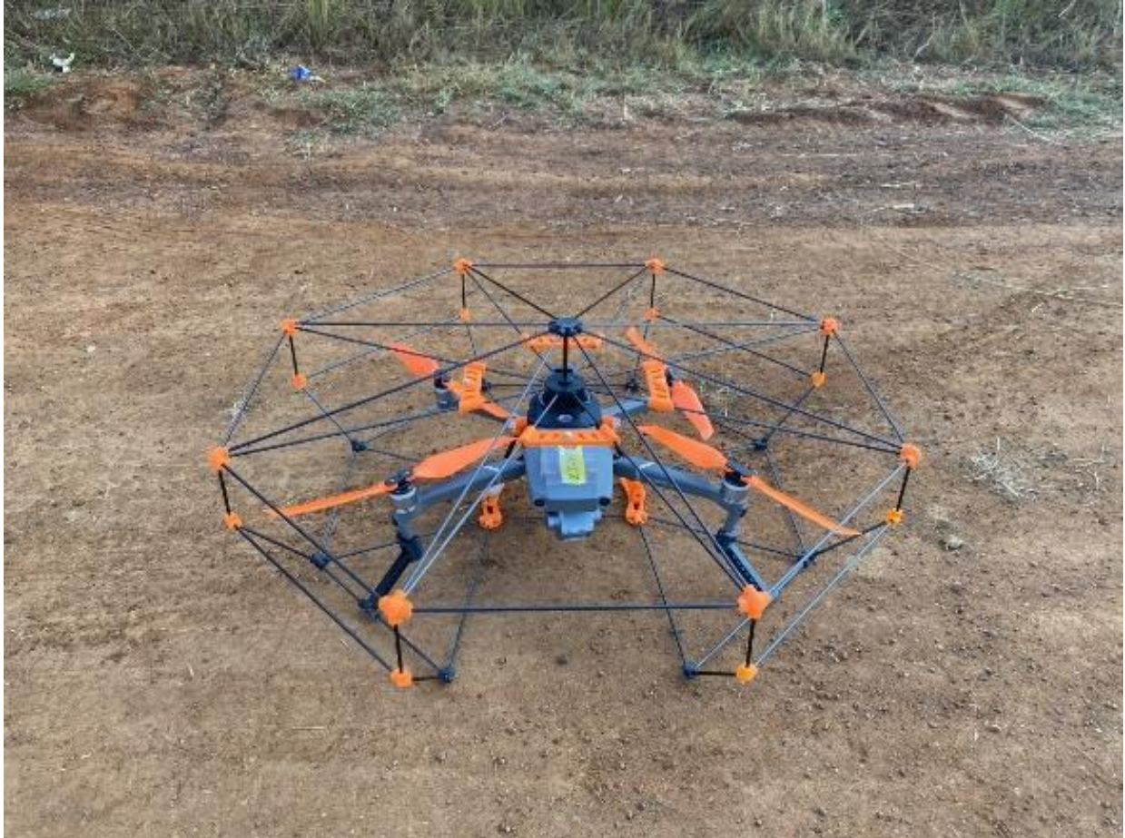
Figure 2-1: Mavic 2 Pro UAV with a protective cage
