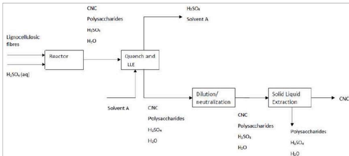
Fig. 3. Domtar Corporation CNC production schematic (Marcoccia et al., 2016).
