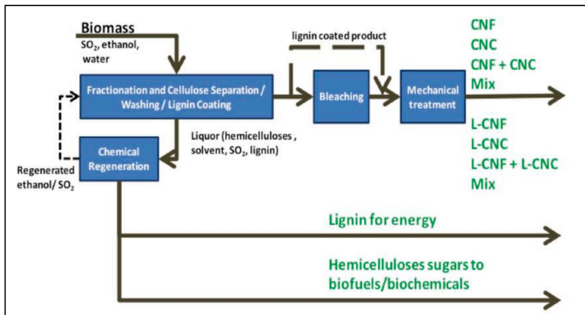
Fig. 1. Schematic of CNC production used by American Process Inc. (Nelson and Retsina, 2014)
