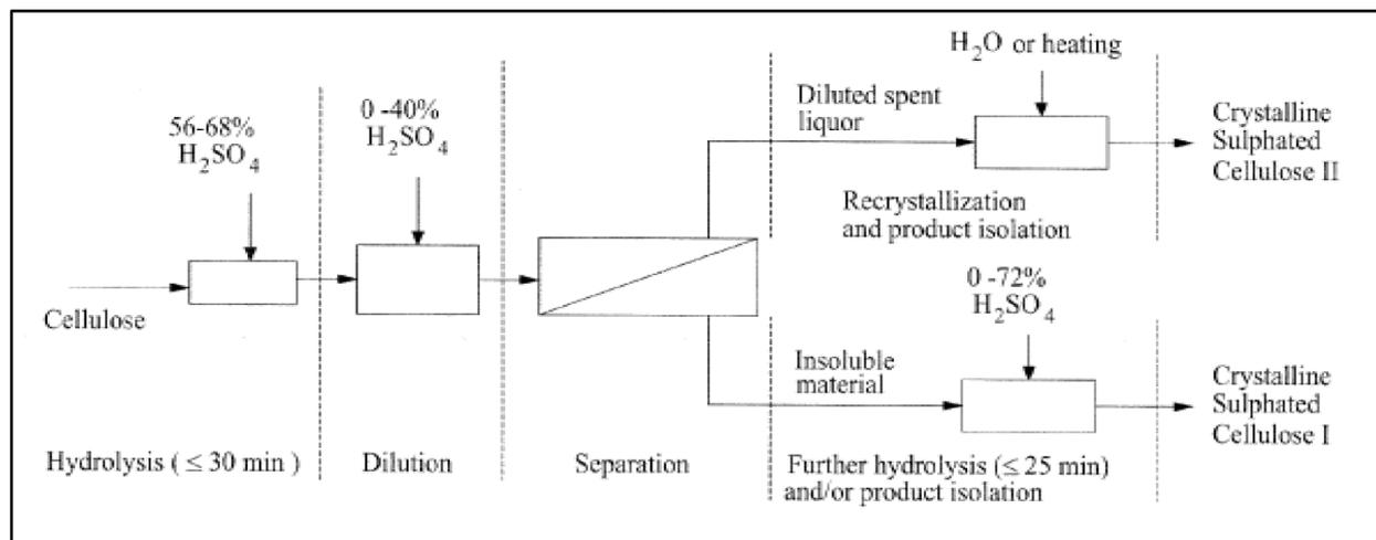
Fig. 4. CNC production schematic at FPInnovations (Hashaikeh et al., 2010).
