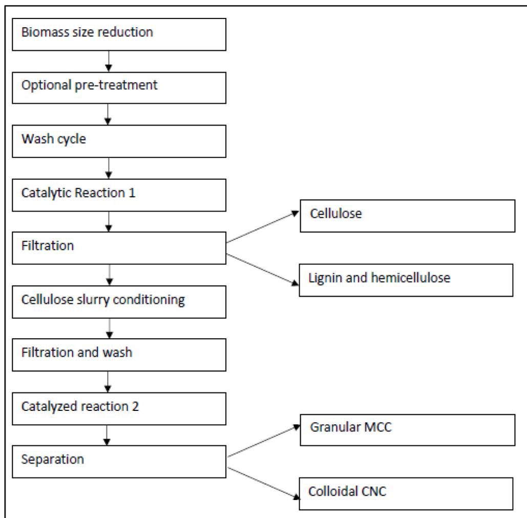
Fig. 5. Catalytic biomass conversion at Nano Green Biorefineries Inc. (McAlpine and Koneshny, 2017).
