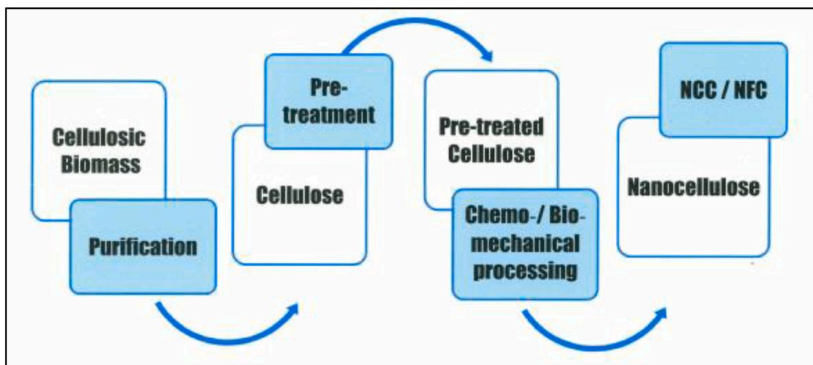
Fig. 2. Schematic of ICAR-CIRCOT CNC production process ("ICAR- Central Institute for Research on Cotton Technology," n.d.).
