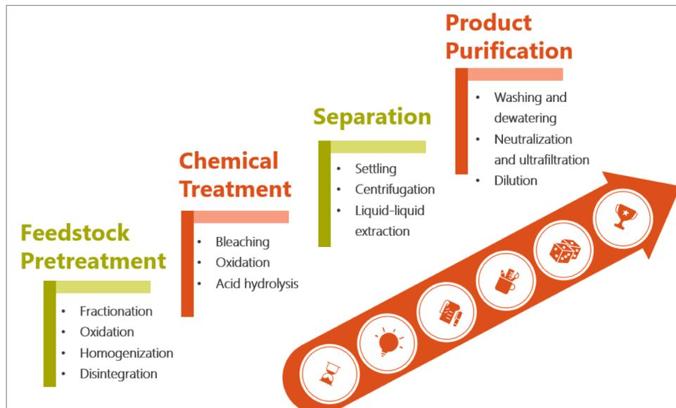
Fig. 8. The four main segments of CNC production.
