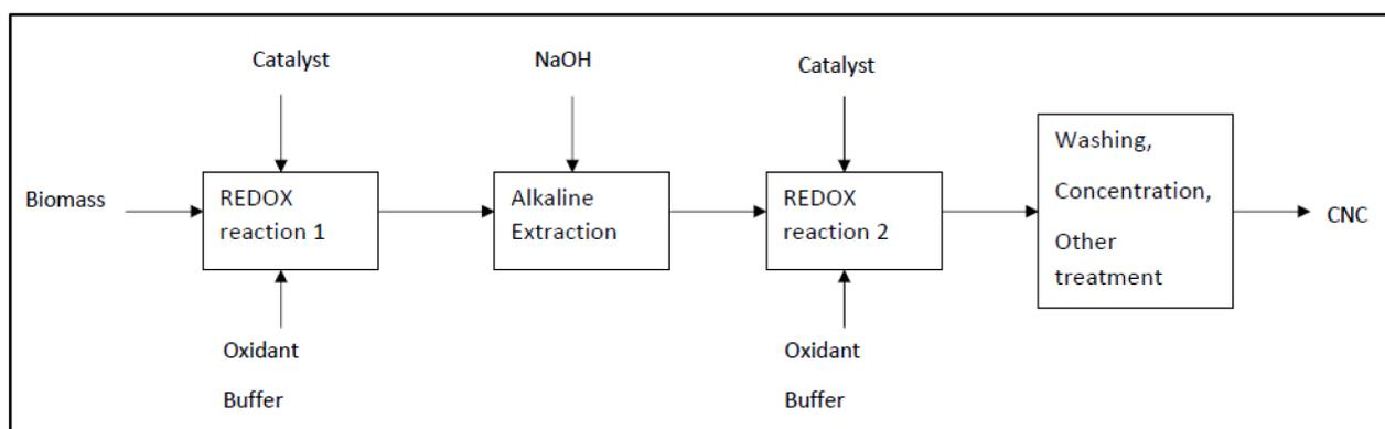
Fig. 6. CNC production schematic at Nano Green Biorefineries Inc. (McAlpine and Koneshny, 2017).
