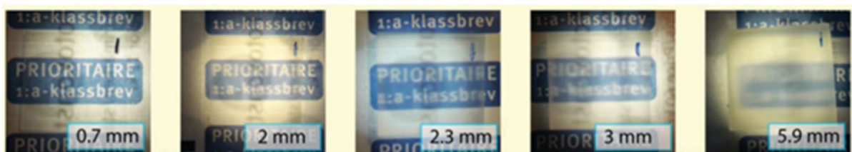
Fig. 3 Photographs of ETW of varying thickness. Reproduced with permission Copyright 2018, John Wiley and Sons (Vasileva et al. 2018)
