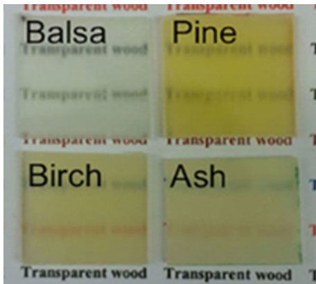
Fig. 4 Images of ETW produced from balsa, pine, birch, and ash. Reproduced with permission Copyright 2017, John Wiley and Sons (Li et al. 2017a)
