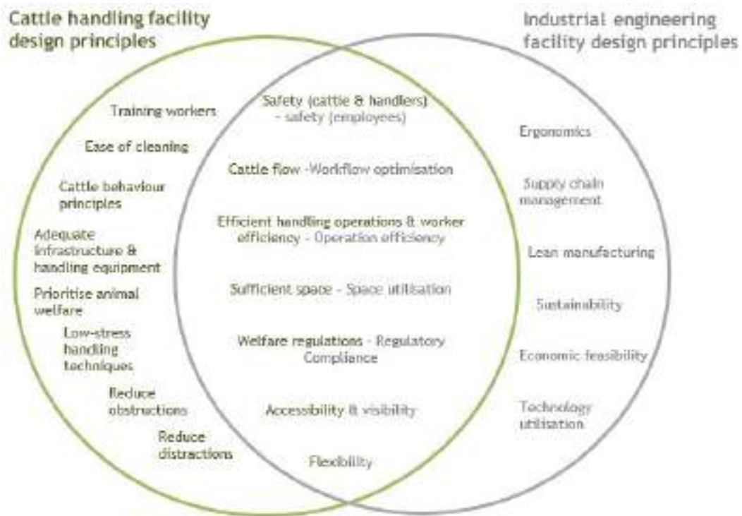
Figure 4: Venn diagram of correlations and variations between industrial engineering- and cattle handling facility design principles
