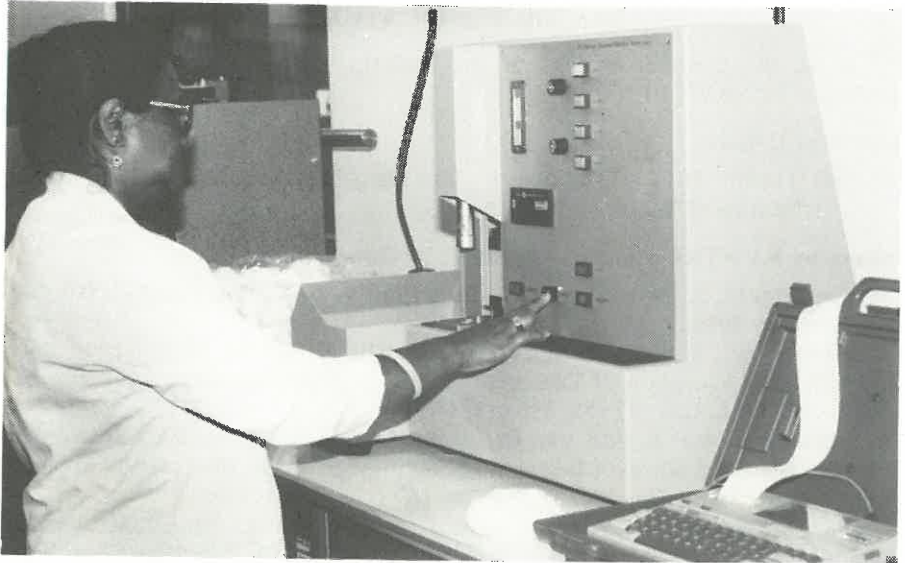
The IIC Shirley Fineness Maturity Tester recently acquired by SAWTRI.
