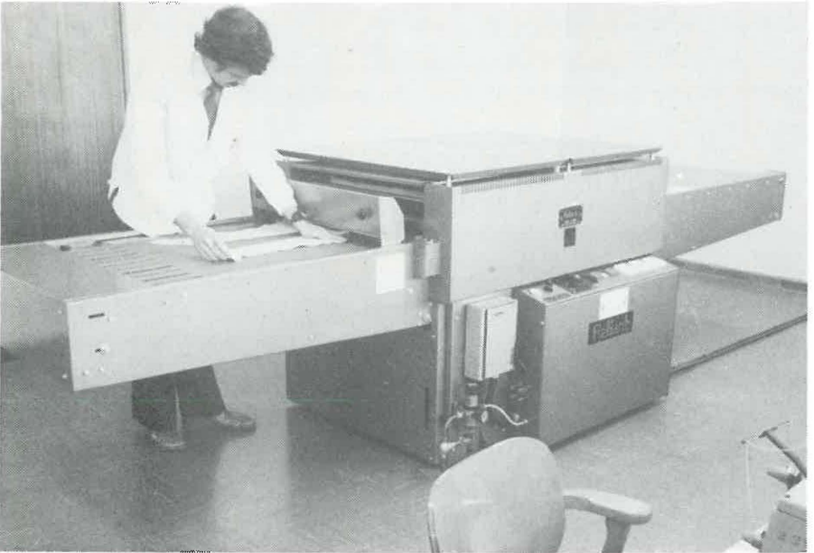
SAWTRI's Clothing Technology Division recently had a Reliant fusing press installed. Here Mr Mike Cawood, Head of the Division, prepares some interlinings for fusing.
