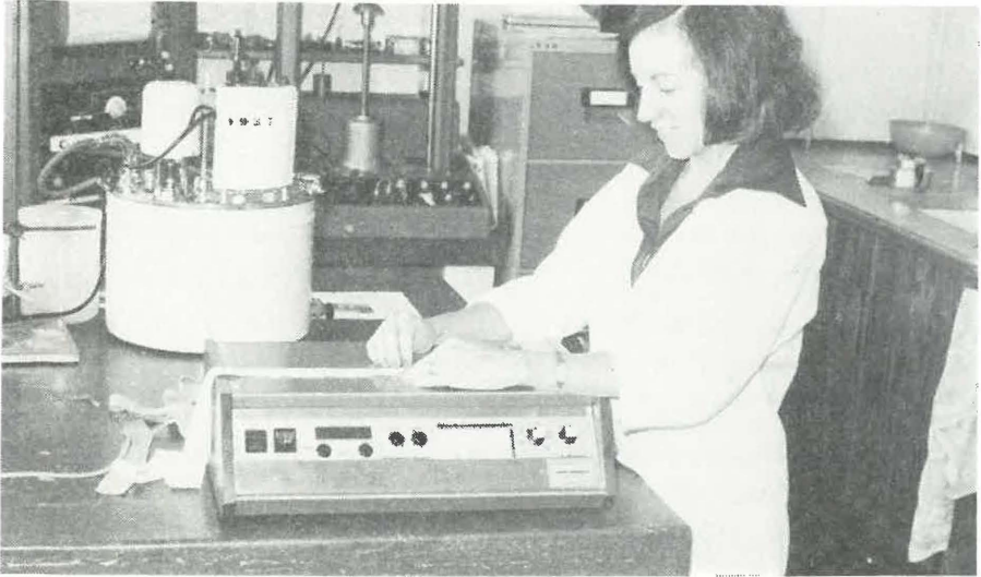
The Textile Physics and Testing Division's new L & M sewability tester for measuring forces generated during sewing
