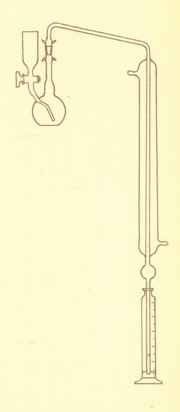
FIG. 2. DISTILLATION APPARATUS.
