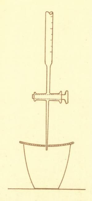
FIG. 1. DECOMPOSITION OF THE MELT WITH SULPHURIC ACID.
