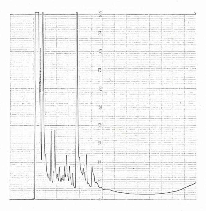
FIGURE 21. Gas chromatogram of the gases formed by a coal dust explosion in the Hartmann bomb.
