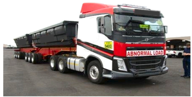
Fig. 2. 74-t interlink transporting coal in the PBS pilot project.
