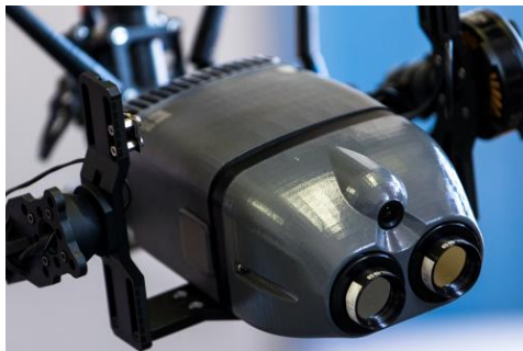
Figure 3: NIR sensor consisting of two cameras side by side furnished with ultra-narrow filters.
