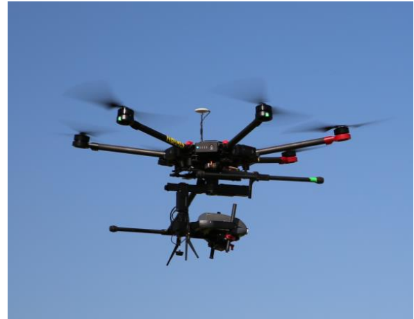
Figure 4: UAV with NIR sensor payload on the DJI 600 drone during a field testing of the sensor.
