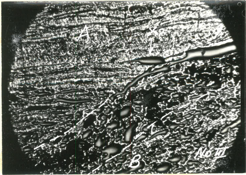
Photomicrograph No. III. (No. 5 Seam char) (Mag. 25X) Showing the nature of the cells and cell wall substance of the zone cementing pieces A and B together.
