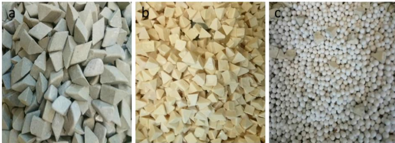
Fig. 1: Different sample media (a) ceramic media angle cut 10X10mm, (b) plastic media pyramid cut 6X6mm, (c) zirconia balls 4X4mm mixed with ) plastic media pyramid cut 6X6mm
