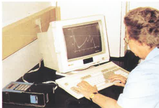
The radiation spectrometer for environmental monitoring. The instrument has been designed to measure all types of radiation underground and to log all relevant information. This information is retrieved and analysed using computer software being specifically developed for the purpose.
