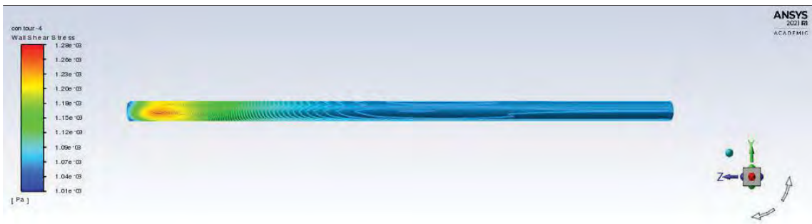
Figure 4 Contours of wall shear stress inside a 200 mm diameter distribution pipeline
