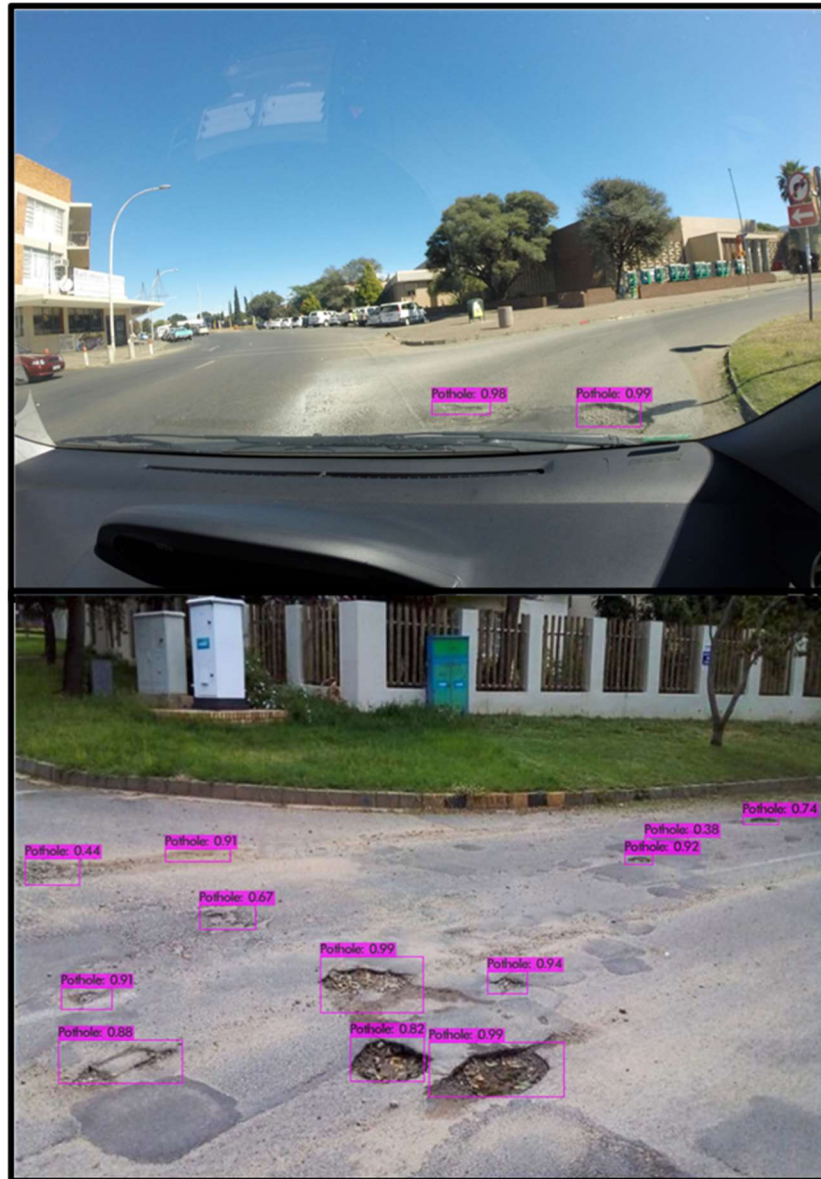
Fig. 7. Detections of potholes using retrained YOLOv3
