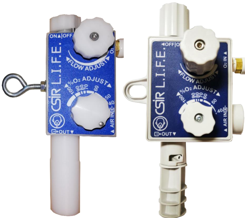
Fig. 7. CSIR L.I.F.E. CPAP, CNC (left) vs. Moulded (right) model
