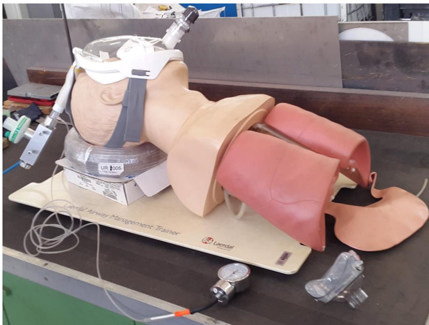
Fig.10. Ventilator and mask testing against test dummy
