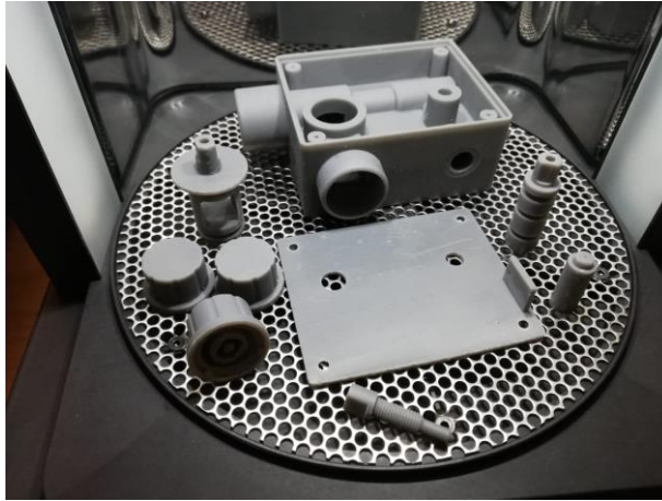
Fig. 8. Printed parts produced by the resin printer
