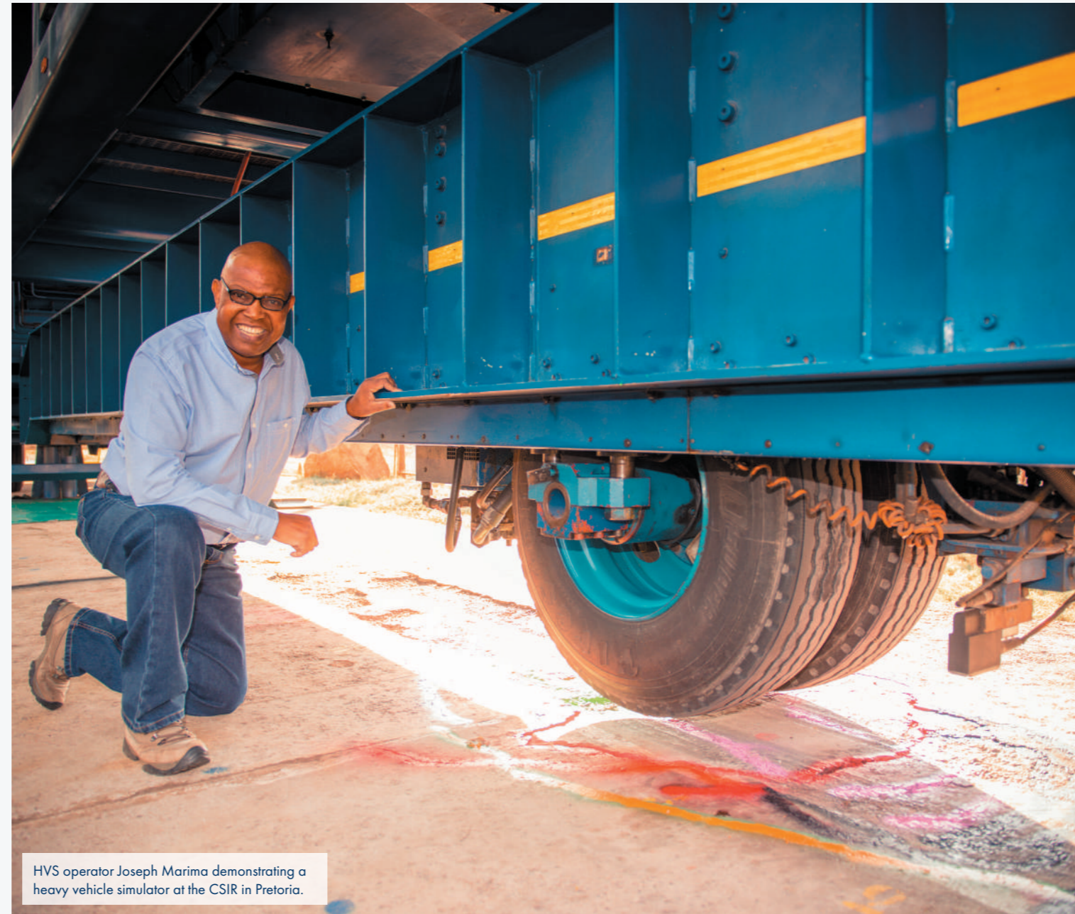
Heavy vehicle simulators such as those used by the Gauteng Provincial Department of Roads and Transport, simulate the dynamic loading effects of trucks on a road and evaluate the structural response.
