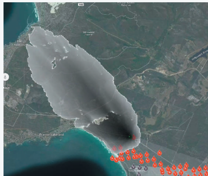
A simulated fire scar in a populated area between De Kelders and Pearly Beach in the Overberg region in the Western Cape. AFIS is valuable in predicting how a fire is likely to spread, assisting authorities with fire suppression strategies and determining whether evacuation may be necessary.
