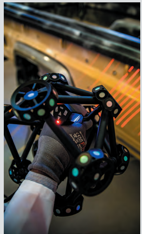
The MetraScan 750 Optical elite scanner is used to scan a Toyota Land Cruiser. This scanner performs highly accurate and repeatable metrology-grade measurements and 3D geometrical surface inspections to create 3D models of objects. Top (right): A bird's eye view of the Advanced Design and Manufacturing Innovation Centre.
