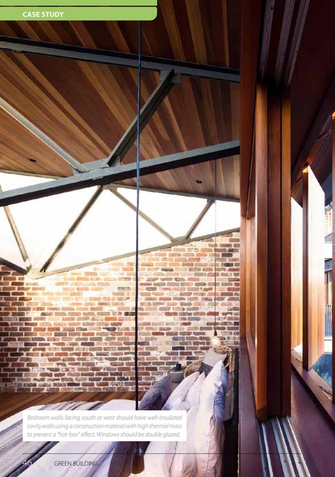
*Bedroom walls facing south or west should have well-insulated cavity walls using a construction material with high thermal mass to prevent a "hot-box" effect. Windows should be double glazed.*
