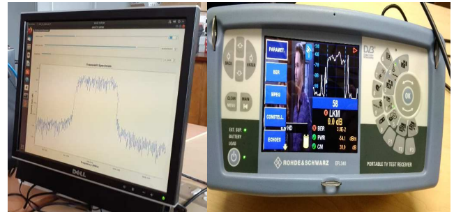
Figure 7: (Left) Digital TV signal scanned on channel 58 by the LCSM node and (Right) TV test receiver also on the same channel
