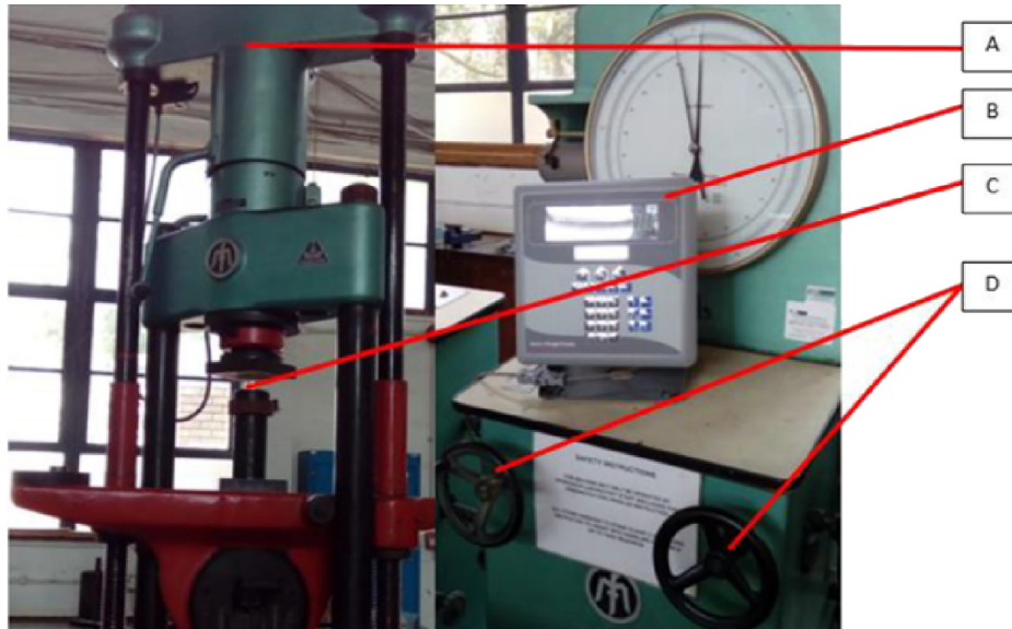
Fig. 3. Compressive strength equipment; A- Tensile testing machine, B- Load indicator, C- base plate, D- Load exertion controls.
