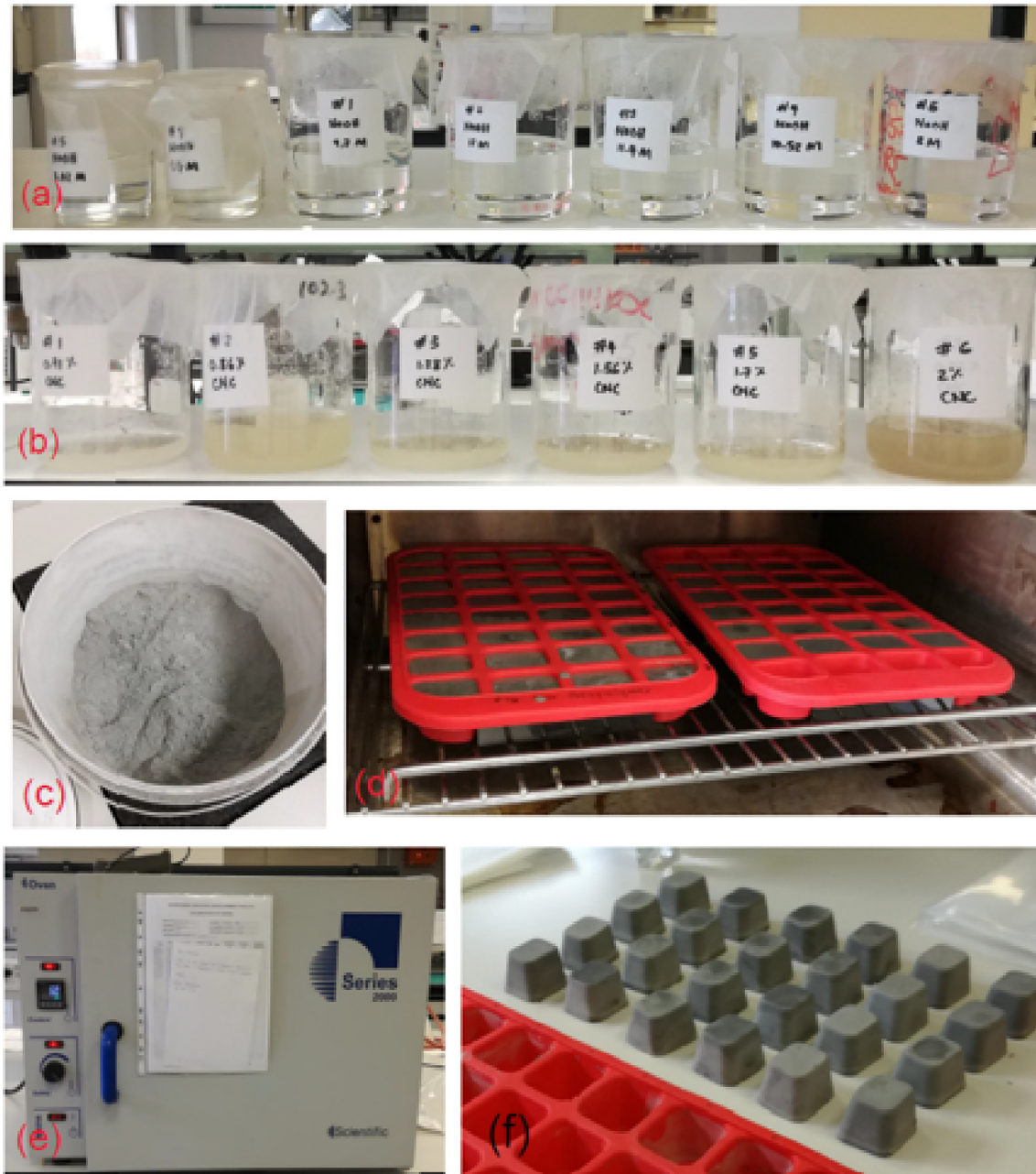
Fig. 2. (a) Alkaline activator solutions (b) Cellulose nanocrystals solutions (c) Fly ash (d) Moulded geopolymer pastes prior to curing (e) Oven used for curing (f) De-moulded geopolymers post-curing.
