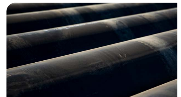
The CSIR-developed coating material (above) used by Hall Longmore to coat its steel pipes (below).
