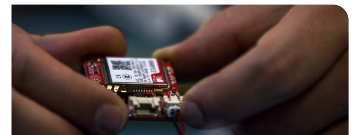
Above: Components of the CSIR-developed device that monitors indoor carbon dioxide levels and generates an alarm when corrective action is needed.
