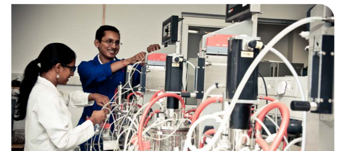
Above: Dr Ghaneshree Moonsamy and former colleague Arvesh Parsoo set up lab-scale bioreactors to conduct microbial cultivations.
