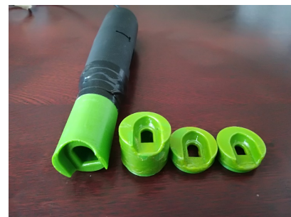
Figure 11. The contactless infant fingerprint acquisition device with different sized attachments to cater for varying sizes of children's fingers
