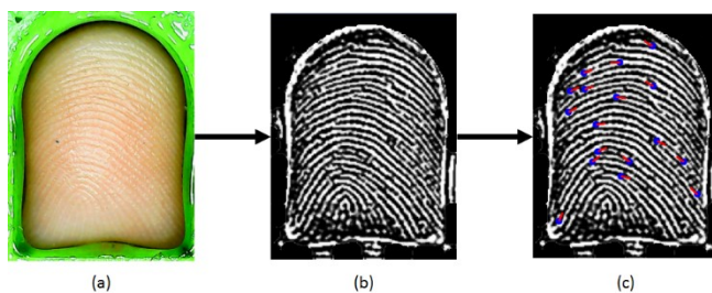
Figure 13. An illustration of the process from (a) the acquisition of the image of an infant's fingerprint, to (b) image processing to convert the fingerprint into a format which is compatible with commercial off-the-shelf comparison software, to (c) the extraction of minutiae points from the fingerprint.
