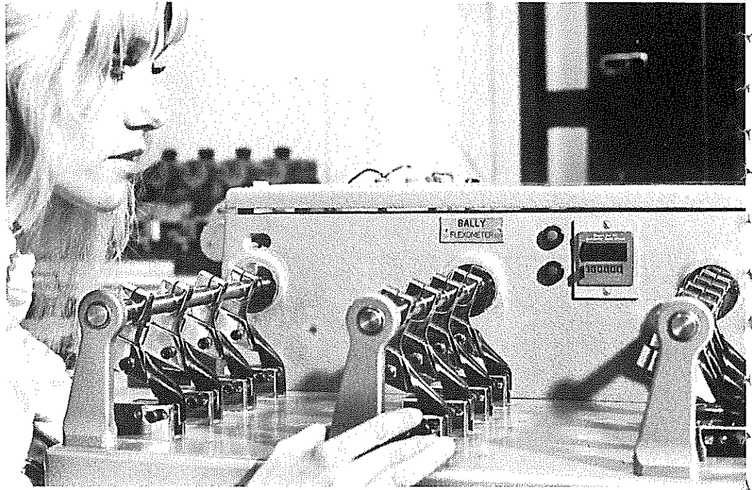
The quality of footwear upper materials being tested on a flexing machine at the Leather Industries Research Institute (p. 26).
