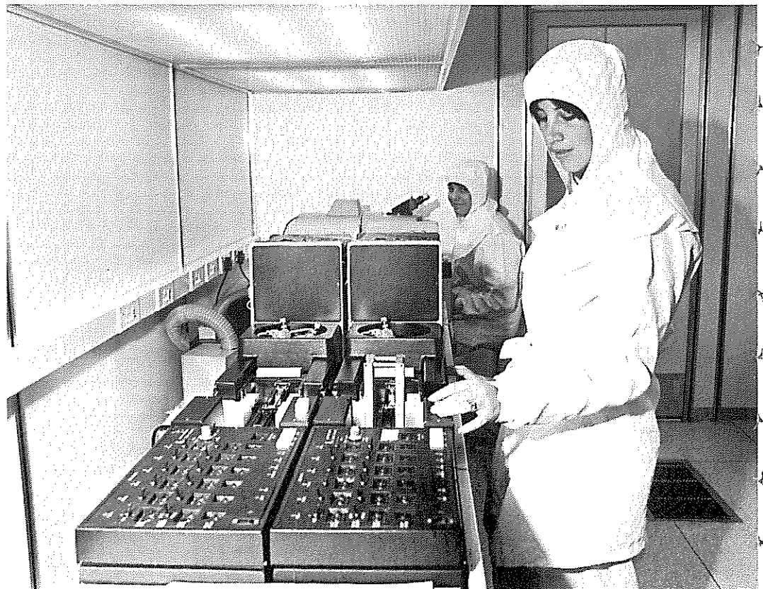
The manufacture of specialised microcircuits at the CSIR's integrated circuit production facility for the local electronics industry (p. 29).
