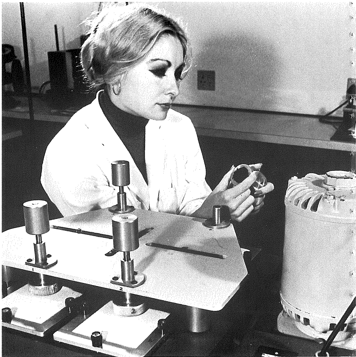
Measuring the abrasion resistance of the fur on Karakul skins as part of the quality control procedures developed at the Leather Industries Research Institute (p. 26).
