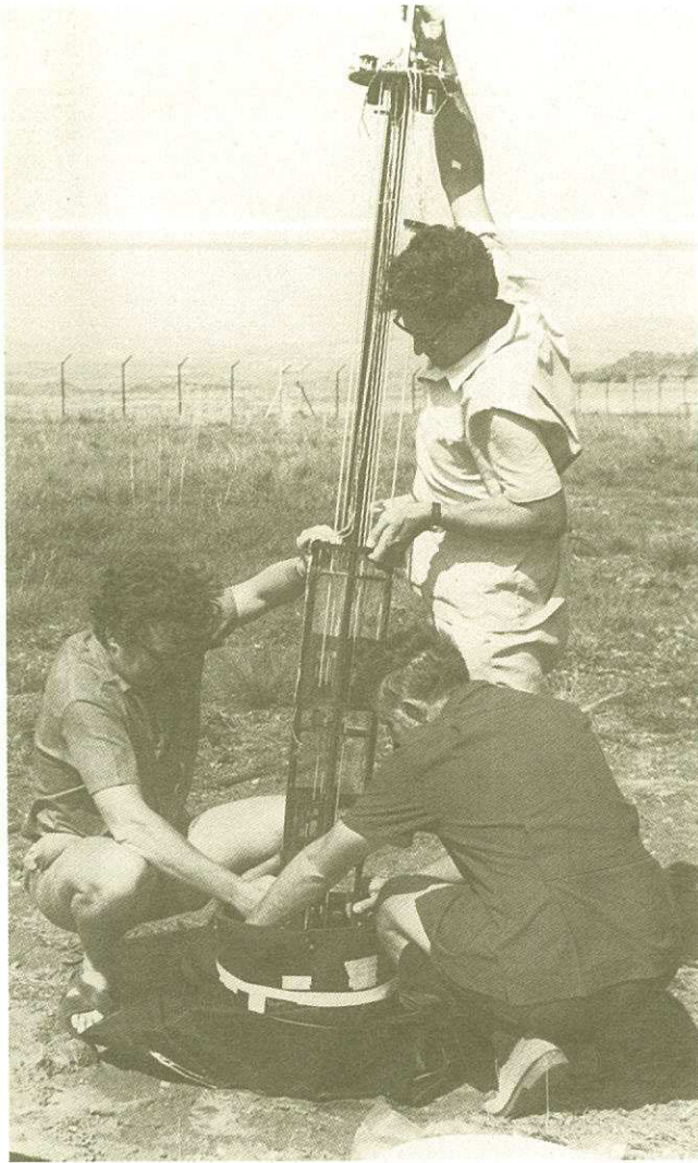
Installing a magnetometer sensor at the Hartebeesthoek recording station.
