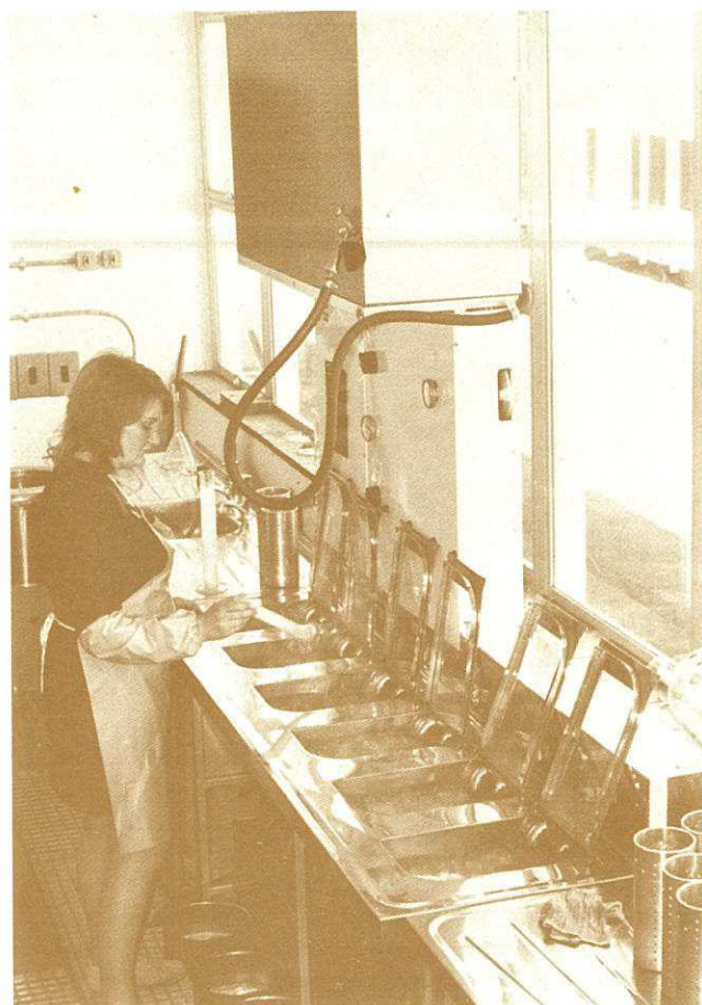
Wool samples being washed in the New Zealand six-bowl scourer to determine clean yield. This is standard procedure in the objective evaluation of the South African wool clip.
