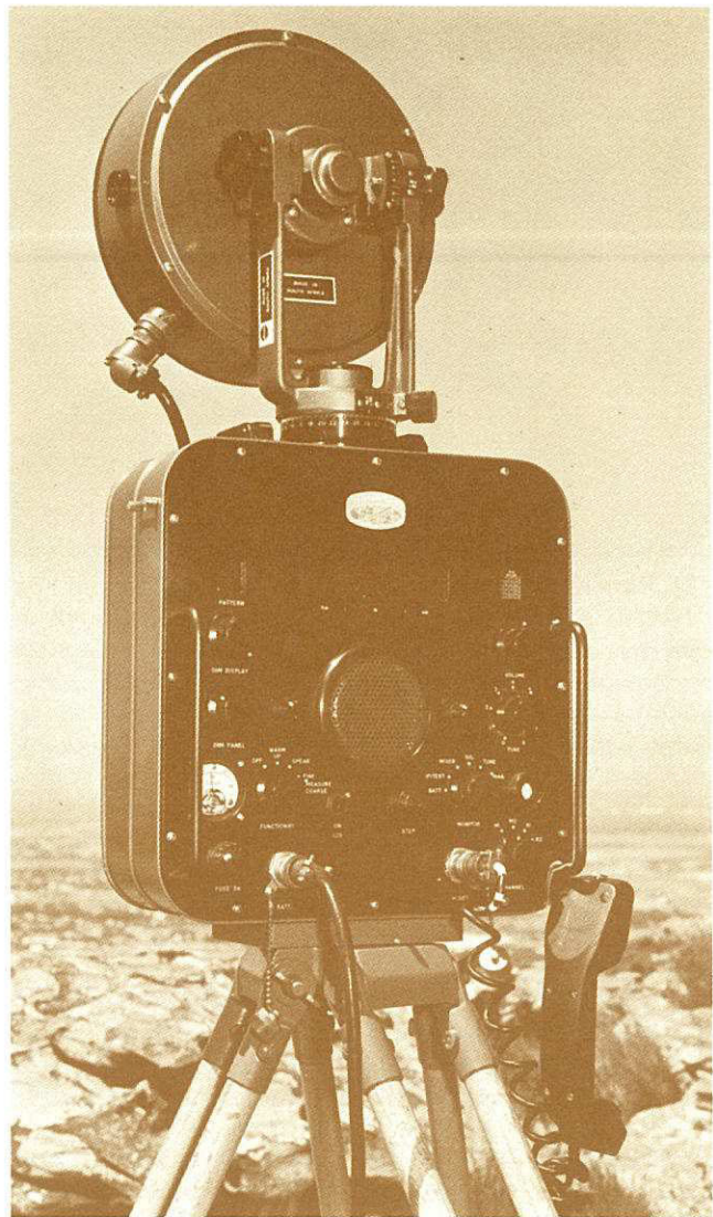
Prototype automatic 'Tellurometer' distance measuring equipment. Below, tests are being conducted with the antenna unit elevated on a mast.
