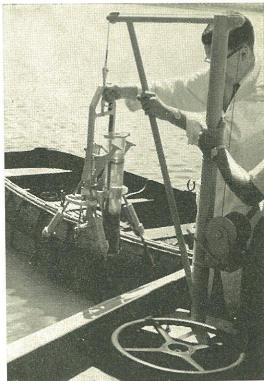
A Jenkins sampler being used in the study of bottom sediments in rivers and dams.
