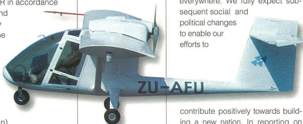
Developed by the CSIR, an all-composite two-seater turbo-prop aircraft.
