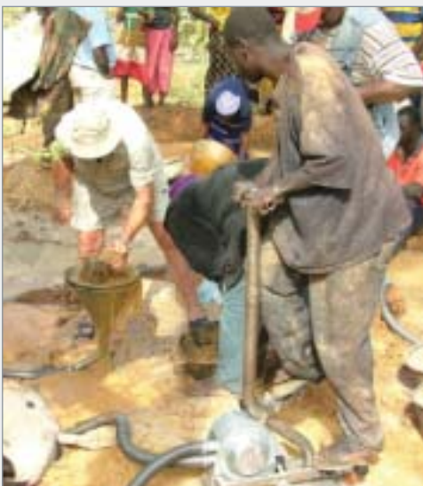
The innovative stepping pump concentrator modified by the CSIR for use by small-scale miners in Africa
