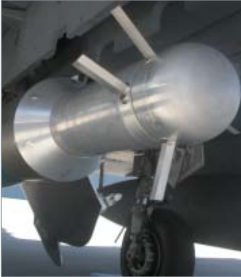
The CSIR has developed novel technology to excite aircraft during flutter flight testing
