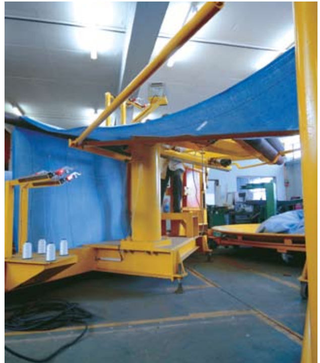
The CSIR, as part of a technology-transfer initiative, developed and patented a helical sewing machine that was given to a backfill bag company.
