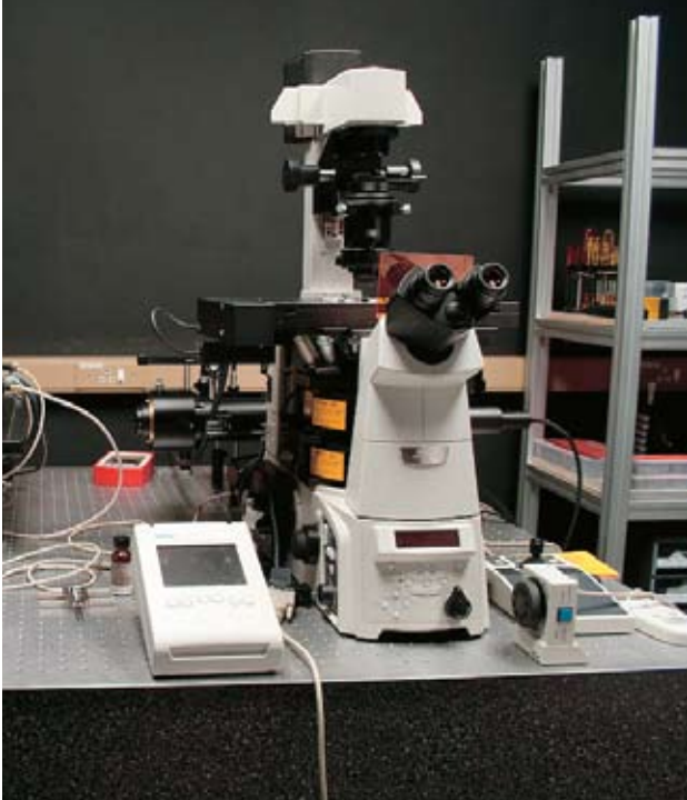
The nanoscopy platform is able to perform routine super-resolution of single biological molecules.
