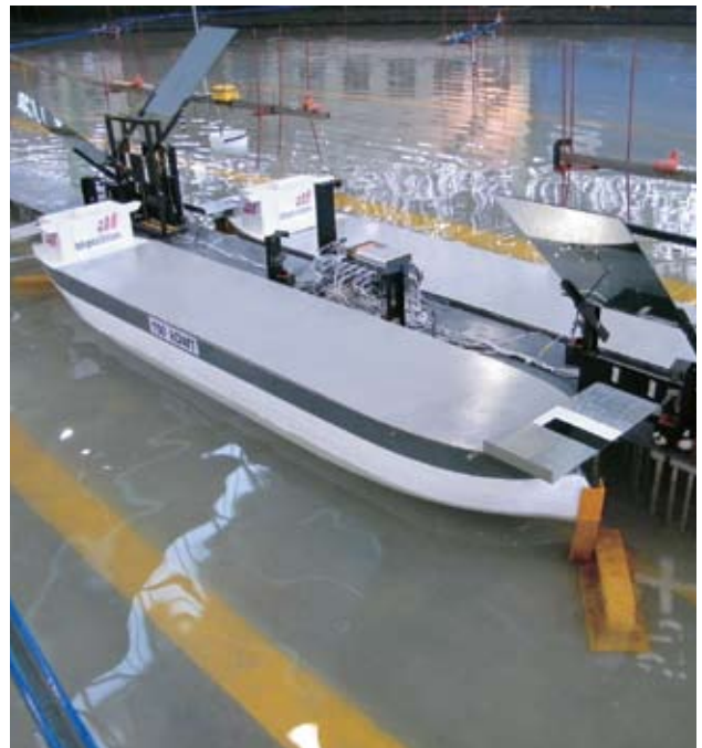
Custom-made model bulk carrier ships were also built for the study.
