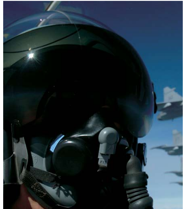
The Cobra helmet, as used in the SAAF's Gripens, can display critical data onto the visor and tracks where the pilot is looking. Images copyright Gripen International.
