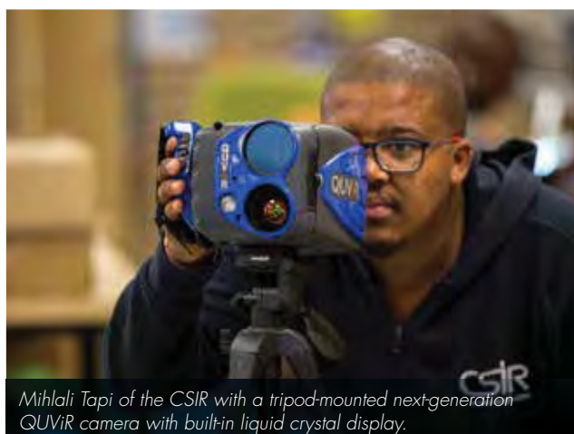
The next-generation QUViR camera: A hand-held multi-spectral imager with fingertip control and viewfinder.
