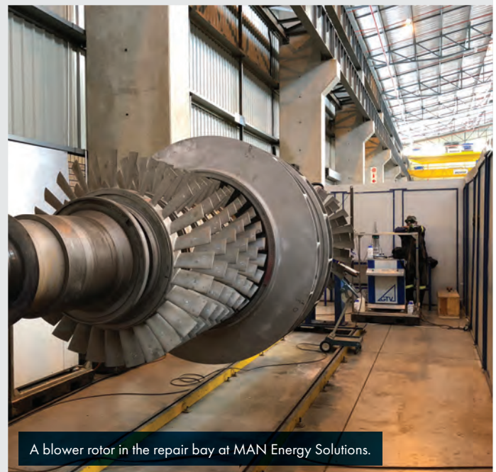
Tip repair of blower rotor blades using laser welding.
