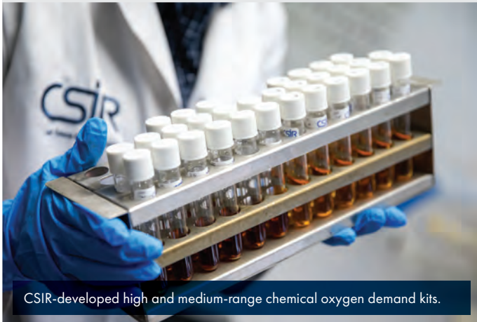
CSIR senior process engineer Prisha Naicker with locally manufactured chemical oxygen demand test kits, developed for a client. Industry and municipalities are required to adhere to water discharge specifications for chemical oxygen demand.
