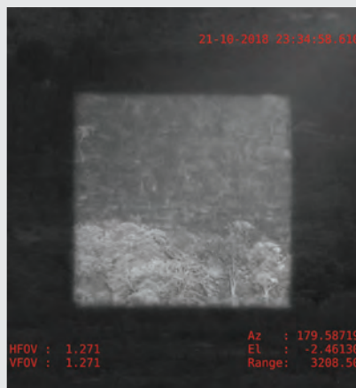
The CSIR has deployed a day-night surveillance camera in the Kruger National Park as part of the Meerkat wide area surveillance system (above). However, operating a coincident sensor-illumination configuration at long ranges when there is high aerosol content in the atmosphere, proved problematic. Following the combination of off-set illumination and optimum laser power, the visibility of objects of interest under low light level conditions improved, as is evident in the image left (below).
