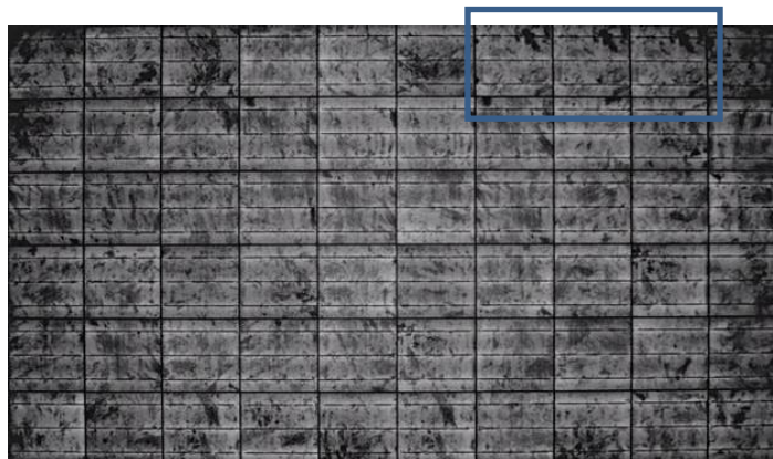
Figure 4.1 EL image of multi-crystalline module with square cells, grain boundaries and three interconnect ribbons.
