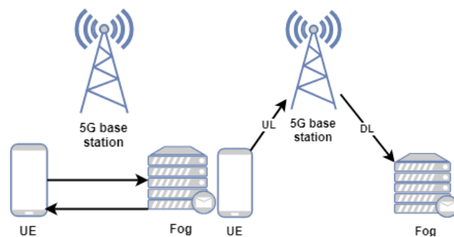
Figure 3: (a) D2D communication (b) Basic access through 5G base station
