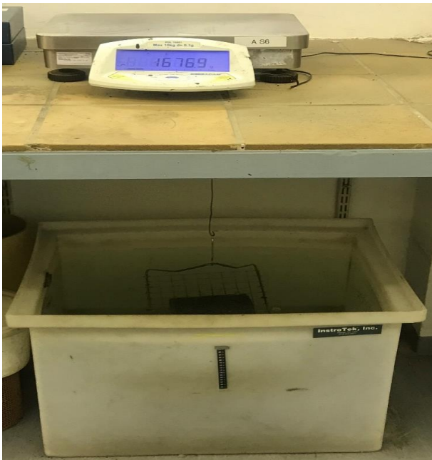
a) Typical SSD set-up
