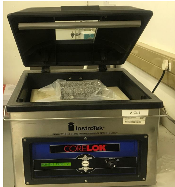
b) Vacuum sealed specimen
