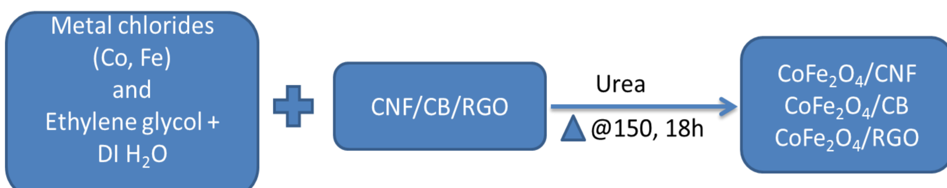
Scheme 1. Hydrothermal synthesis of \text{CoFe}_2\text{O}_4/\text{CNF} , \text{CoFe}_2\text{O}_4/\text{CB} and \text{CoFe}_2\text{O}_4/\text{RGO} materials.
