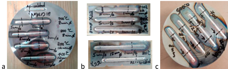
Fig. 2. Single clad tracks and heat treatment runs on a) 21CrMoV5-11, b) X22CrMoV12-1 and c) 34CrNiMo6 substrates.
