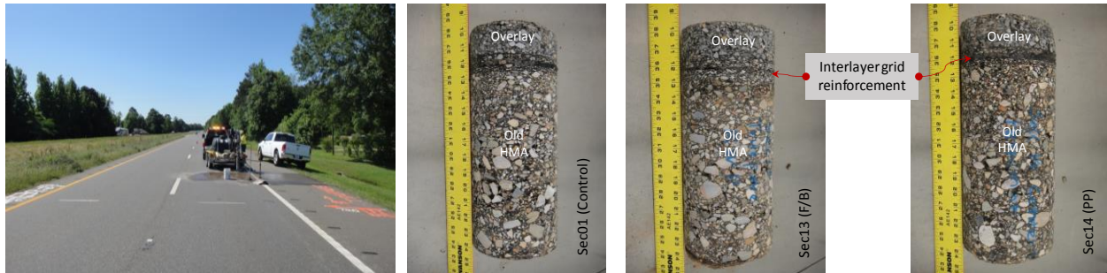
8 9 Fig. 10. Intact and Fully Bonded Cores.
