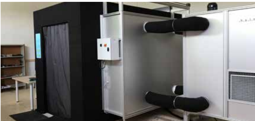
▲ Figure 1: A+A+A+ solar simulator with integrated thermal chamber
