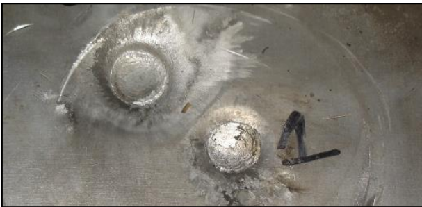
Fig. 11 Indentation test on 16 mm aluminium plate
