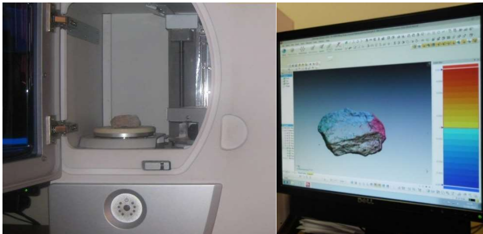
Figure 3. Scanning and modeling of aggregate particles in the 3-d laser scanning system.
