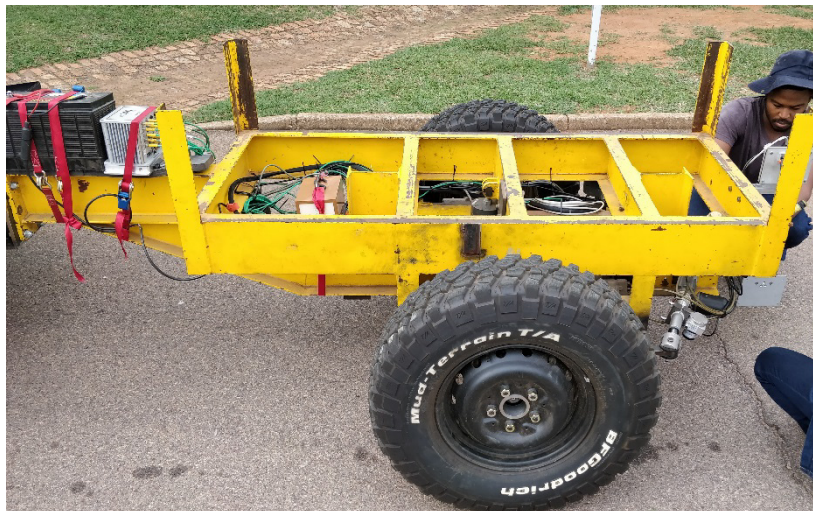
Figure 1: CSIR’s medium-size tyre tester
