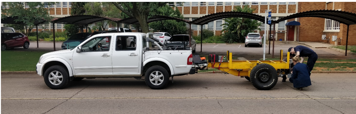
Figure 9: The medium tyre tester and towing vehicle ready for testing
