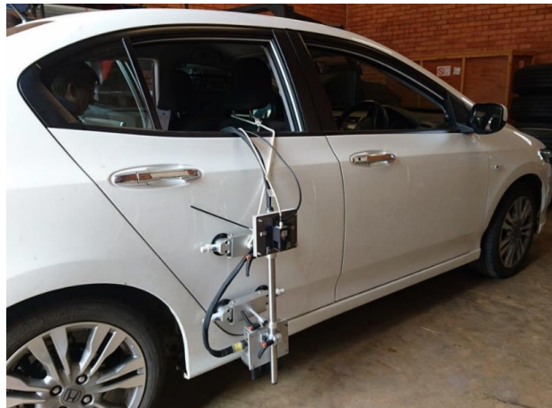
Figure 6: Correvit sensor and camera mounted to the vehicle for validation
