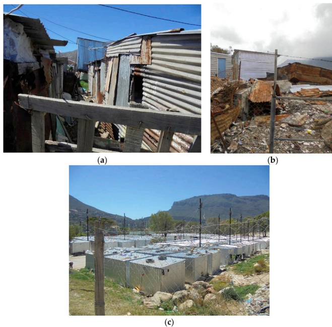
Fig. 1. a) Imizamo Yethu informal settlement in Cape Town illustrating the makeshift nature of building methods and materials, narrow pathways and combustible materials between dwellings, b) collapse of a dwelling due to a fire and c) new dwellings constructed from starter building kits provided by City of Cape Town post-fire.
