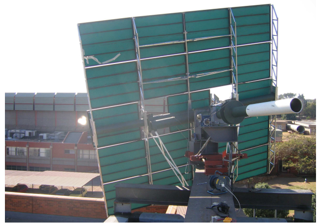
Figure 1: Rear view of heliostat, showing focal spot on wall above stairwell terminal on roof of northern building and parapet wall on roof of southern building in foreground
