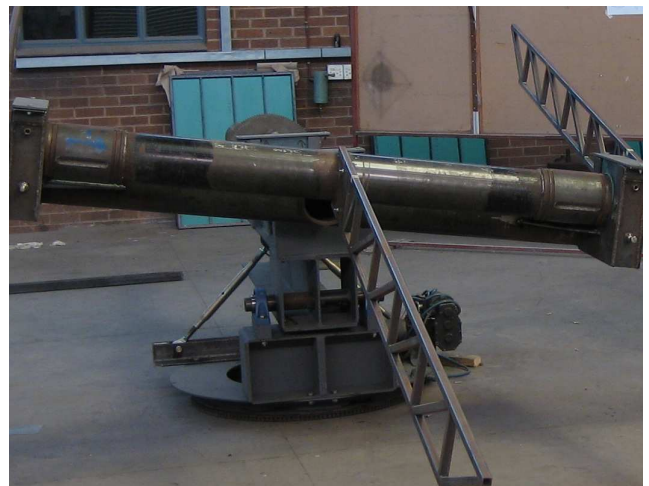
Figure 8: Thrust bearing rings on the pitch axis torque tube, up against the bearings
