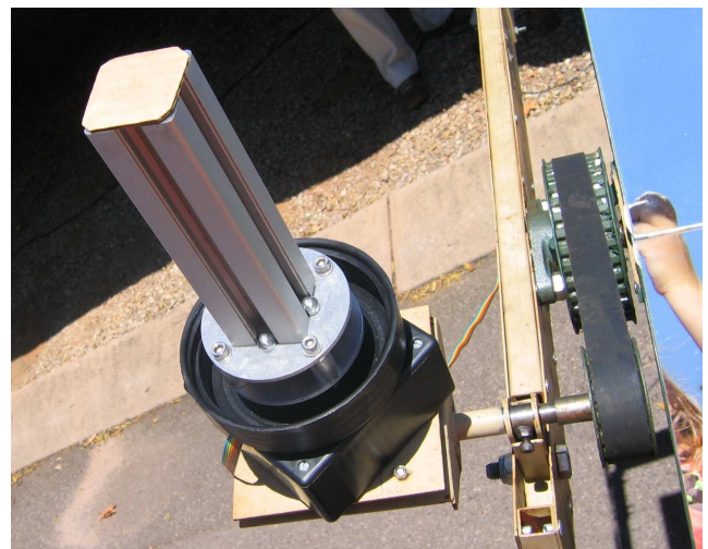
Figure 9: Close-up of solar tracker, geared 2:1 to the pitch axis
