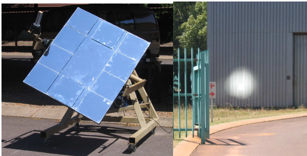
Figure 10: Mini-heliostat with additional mirror tiles and solar tracker, target of A4 paper obscured by focal spot at 120 metres.
