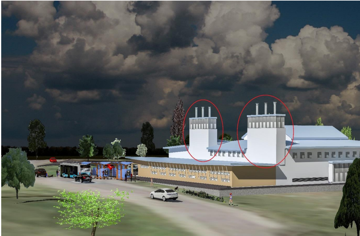
Figure 1: Science centre with the solar chimneys (circled in red) incorporated in the ventilation system (CSIR 2018)
