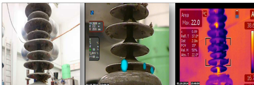
Figure 2: A polymeric insulator inundated with fungus and stressed at 101.5 kV From Left-Right VIS image, UV image and IR image [1]
