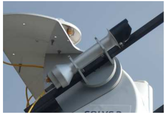
Fig. 5. Pyrheliometer CHP1 mounted on Dual axis tracker at CSIR, Pretoria campus
