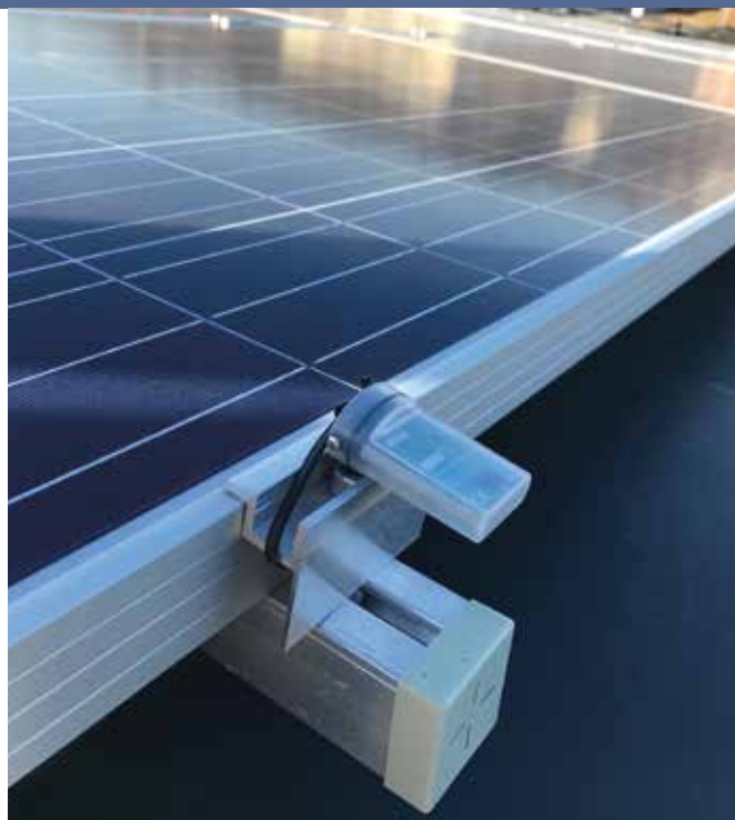
Fig.1 - PV system at Uppsala Science Park used in the UppScaleSolar project with the sensor for solar irradiance measurement (Photo: Joakim Munkhammar).
