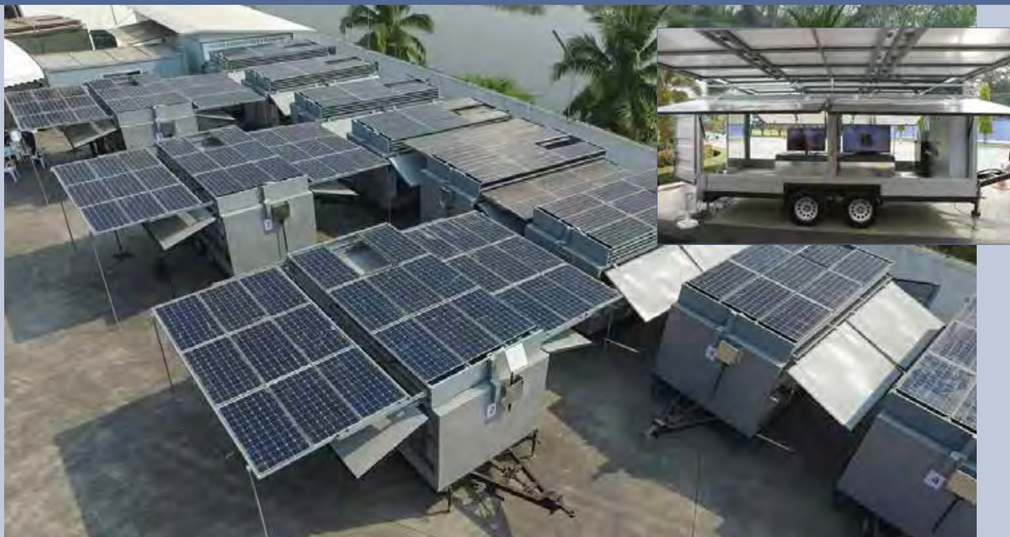
Fig. 1 – The Mobile Solar Cells Trailer Project to Support Electric Power in Three Southern Border Provinces for Military Units and Neighborhoods. Capacity of 6 kW / vehicle, a total of 12 vehicles can replace about 130,000 units of electricity per year, operated by the Internal Security Operations Command and support budget by the energy conservation fund (Photo: DEDE).
